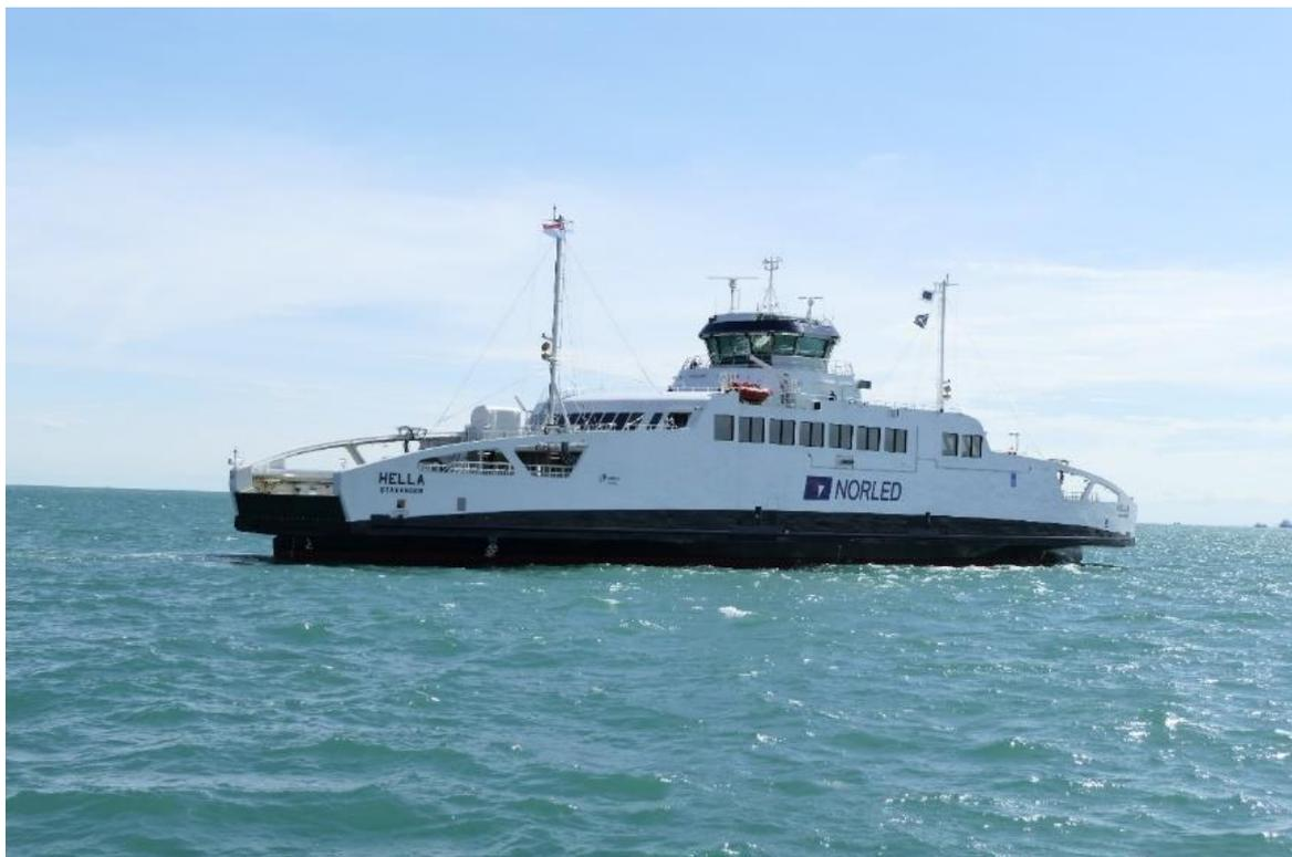
The first of three Norled zero-emission battery-powered Ropax ferries ready for the sailaway to Norway for deployment in the Hella-Vangsnes-Dragsvik service route
