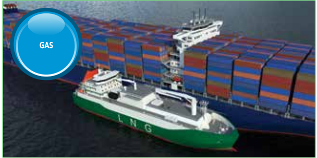
The unique membrane tanks of the 12,000 cbm Liquefied Natural Gas (LNG) bunker vessel, constructed for our customer MOL, will be fabricated under a licensing agreement with LNG containment specialist GTT. This project strengthens our track record in LNG-related engineering designs and solutions.
