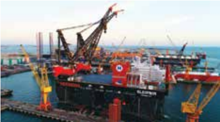
Named after Norse god Odin's eight-legged stallion, Sleipnir 's two main cranes are capable of hoisting 20,000 tonnes in a single lift
