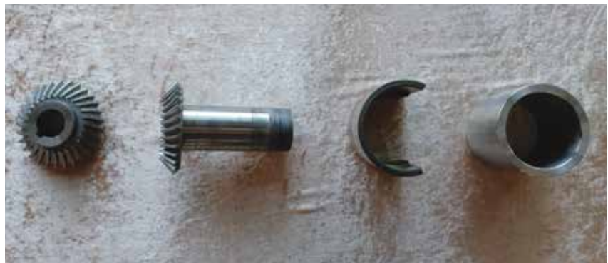
Samples of 3D printed parts certified fit for repair and construction purposes
