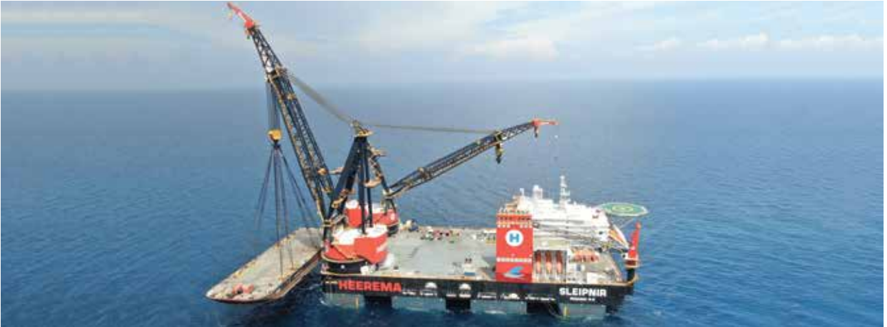
SSCV Sleipnir, delivered to Heerema Marine Contractors in July 2019
