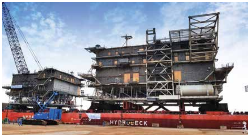
Ørsted's Hornsea 2 wind farm topsides were fabricated at Sembcorp Marine's Batam yard and are now at Admiralty Yard for additional work
