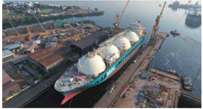
Karmol LNGT Powership Africa undocking from Sembcorp Marine Admiralty Yard after completing FSRU conversion
