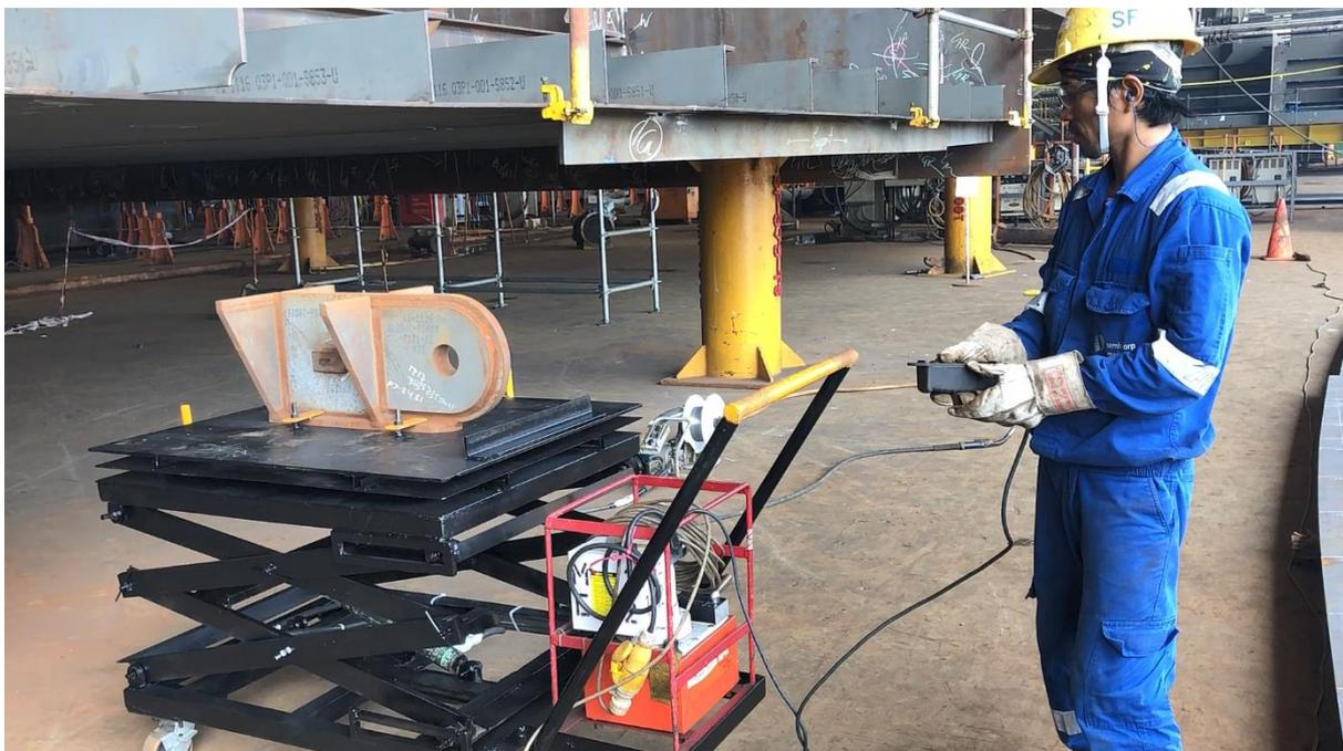
*A Sembcorp Marine worker operating the Eye Pad Arrangement System (EPAS), which elevates eye pads safely for welding onto fabricated structures. Previously, up to four workers were required to perform the welding task, as the eye pad had to be manually lifted and supported during the welding. With the EPAS, one worker can now complete the task on his own.*
