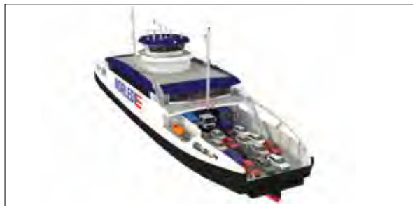
Artist's impression of the Norled hybrid plug-in ropax ferry, which will run on zero-emissions battery power during normal operations
