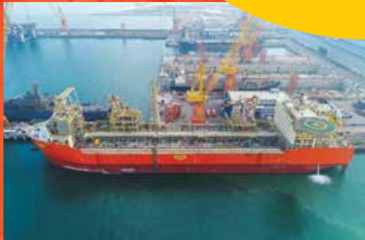
FSO Alisa, the world's first Floating Storage and Offloading vessel with a 40-year hull lifespan, is capable of operating 25 years continuously without dry-docking
