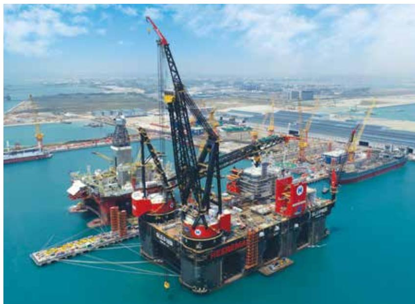
*Heerema's Sleipnir, the world's largest semi-submersible crane vessel (SSCV), undergoing commissioning*
