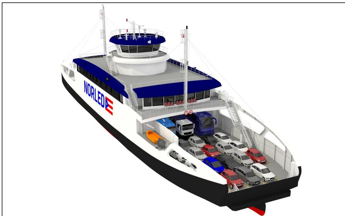
Artist's impression of the Norled hybrid plug-in ropax ferry. Three identical vessels will be completed in 4Q2020 for deployment in the Hella-Vangsnes-Dragsvik service route in Norway. During normal operations, the vessels will run on zero-emissions battery power.
