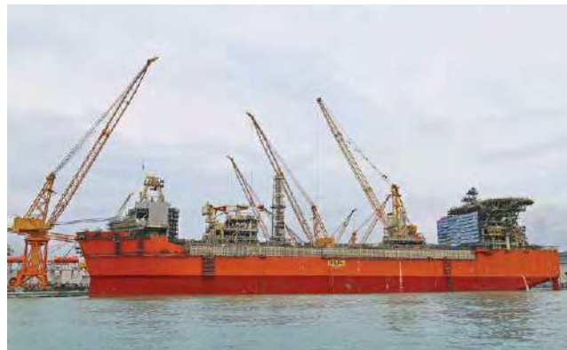
FSO Ailsa is Sembcorp Marine's first turnkey FSO newbuilding project, including Engineering, Procurement, Construction and Commissioning
