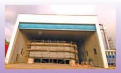
Enclosed blasting and painting chambers limit airborne particles.
