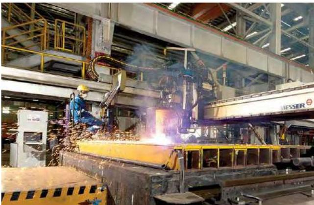
Fuel gases are used to cut and weld steel and other materials
