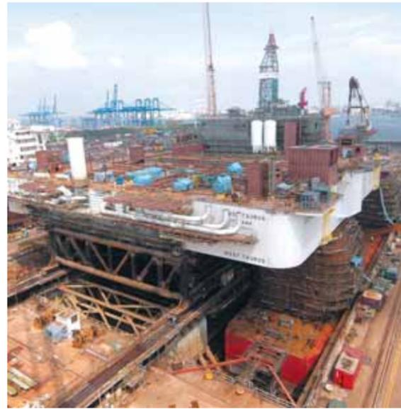
The combination of these two processes enabled multiple rigs to be constructed simultaneously and assembled sequentially in a safe and secure manner at relatively lower cost. The “Transverse Skidding” process further improved on the original “Load-out & Mating-in-Dock” technique which allowed only one semi-submersible to be built at a time.
