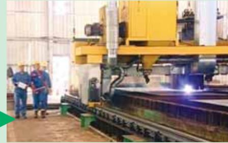
2. Precision cutting of steel plates and components for pontoon fabrication.
